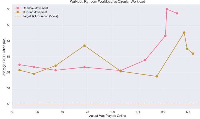
Figure 5.4: Comparison of average tick duration (ms) between the 'random' workload and 'circular' workload
