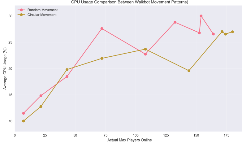
Figure 5.5: Comparison of CPU usage between the 'random' and 'circular' workloads of Walkbot. Small deltas suggest scheduling/contention effects.
