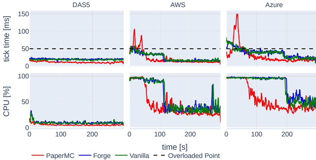
Figure 13: Comparison of tick time and CPU utilization during Internal Variation experiment.
